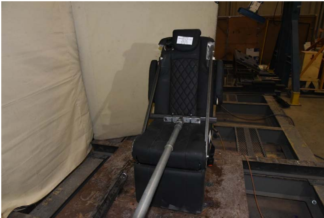
Figure 4: Post-Test Photograph of FMVSS 207 Aft Seat Force
