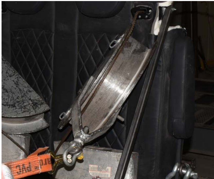
Figure 24: Post-Test Photograph of FMVSS 210 Shoulder Belt Force (Left Side)
