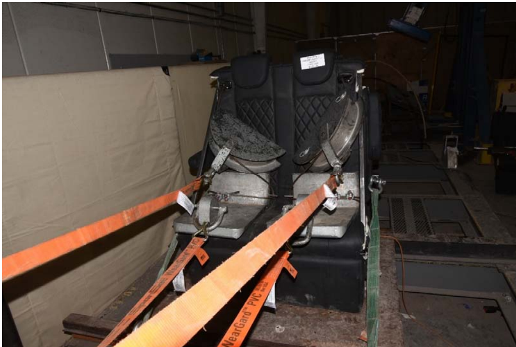
Figure 20: Post-Test Photograph of FMVSS 207 Seat Force
