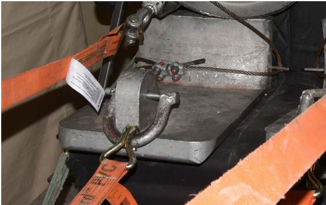
Figure 26: Post-Test Photograph of FMVSS 210 Lap Belt Force (Right Side)
