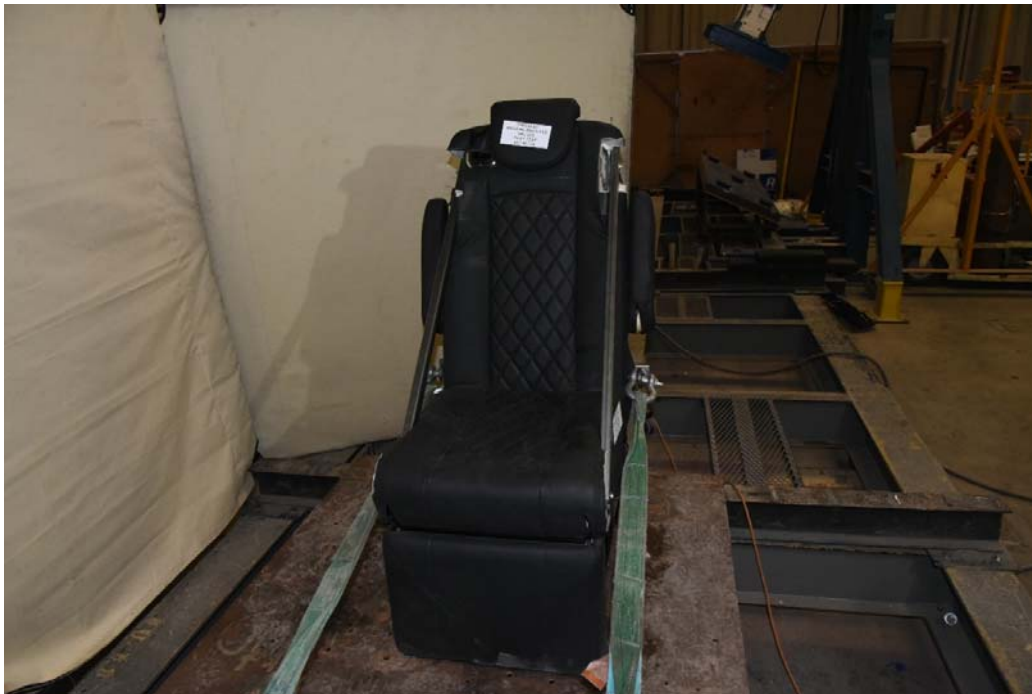
Figure 6: Post-Test Photograph of FMVSS 207 Forward Seat Force
