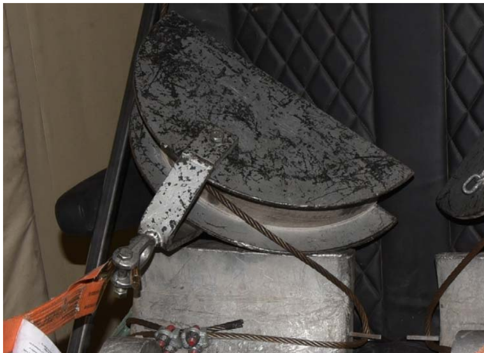
Figure 28: Post-Test Photograph of FMVSS 210 Shoulder Belt Force (Right Side)
