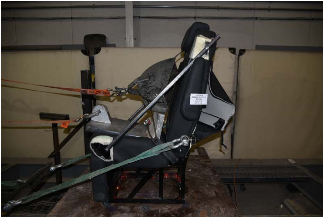
Figure 8: Post-Test Photograph of FMVSS 207 Seat Force
