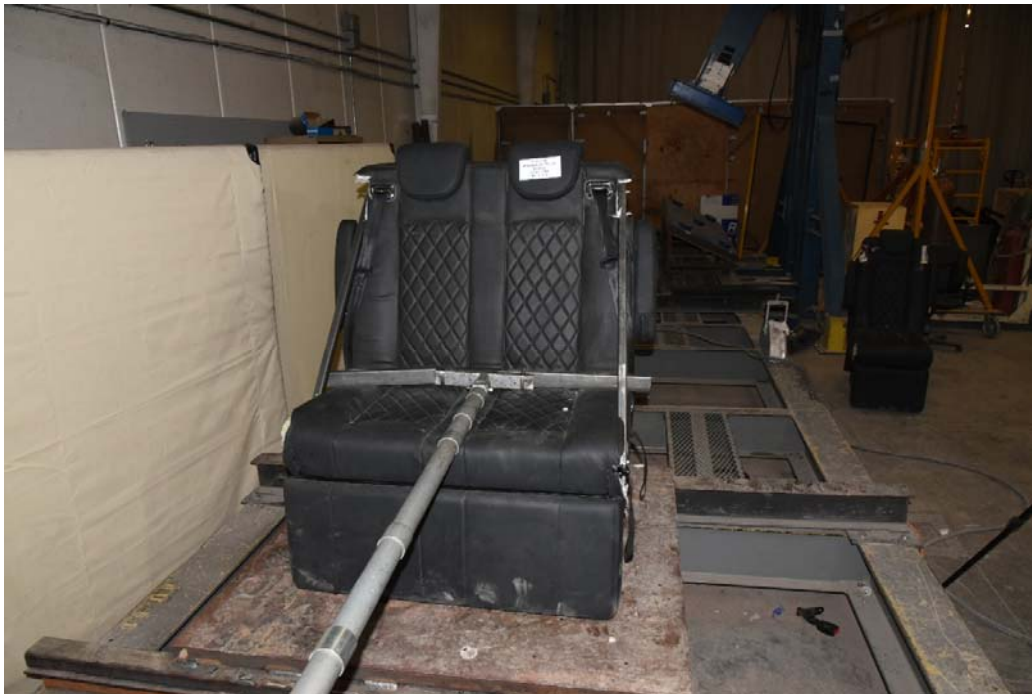
Figure 16: Post-Test Photograph of FMVSS 207 Aft Seat Force
