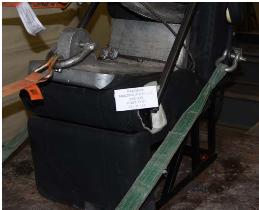
Figure 10: Post-Test Photograph of FMVSS 210 Lap Belt Force
