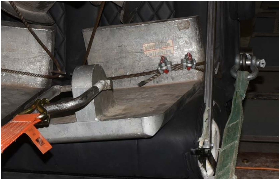
Figure 22: Post-Test Photograph of FMVSS 210 Lap Belt Force (Left Side)
