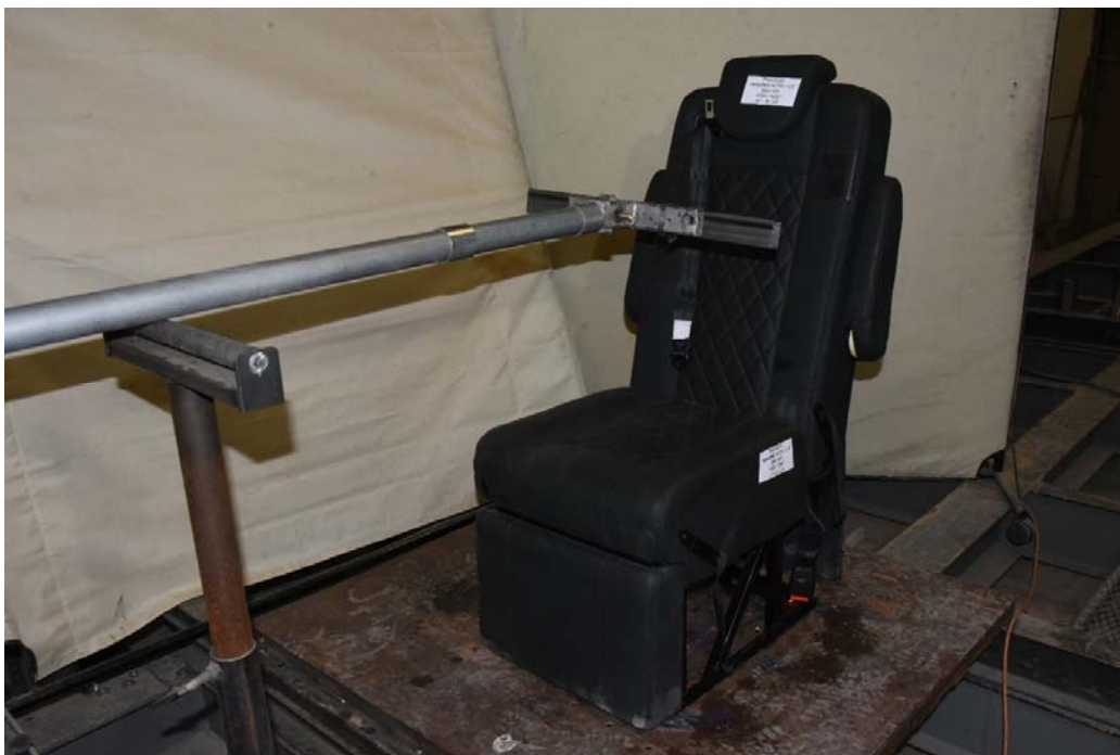
Figure 2: Post-Test Photograph of FMVSS 207 Aft Moment Force
