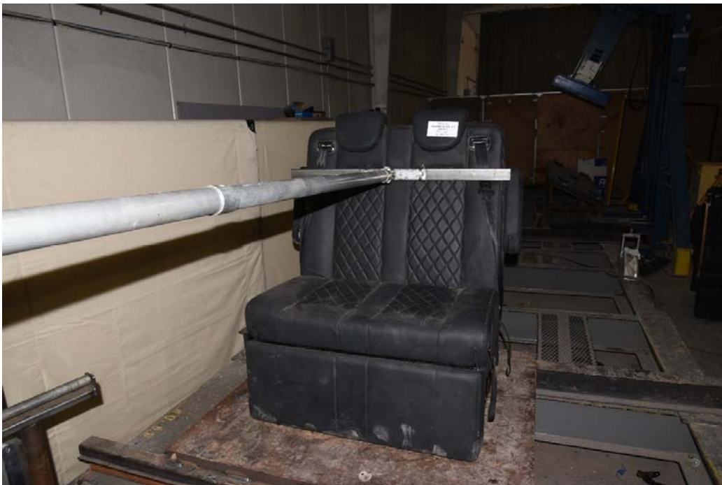
Figure 14: Post-Test Photograph of FMVSS 207 Aft Moment Force
