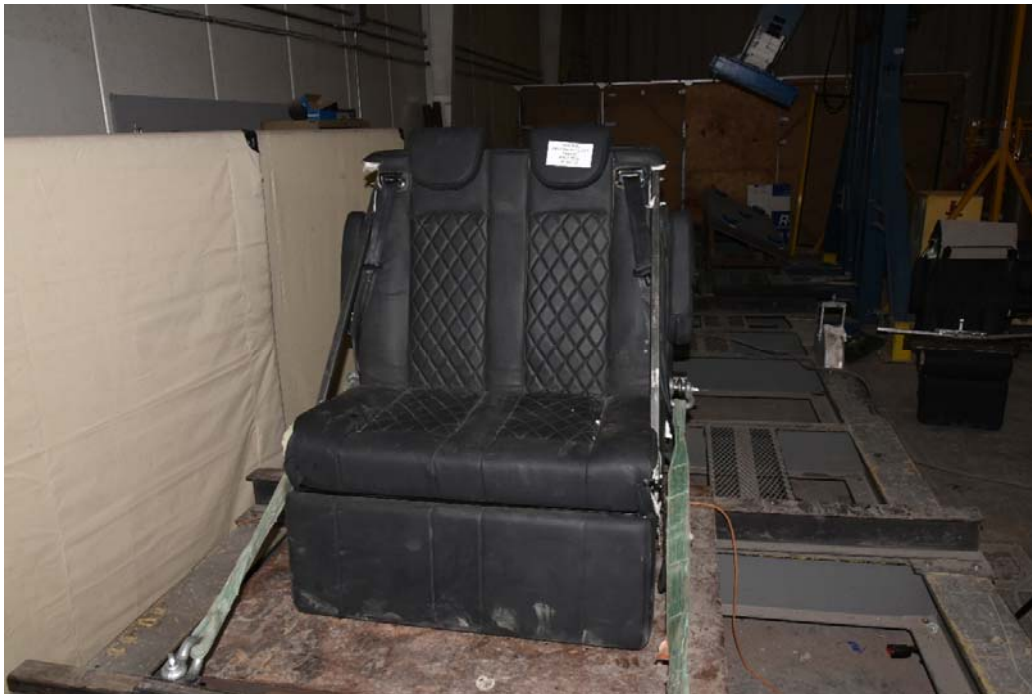
Figure 18: Post-Test Photograph of FMVSS 207 Forward Seat Force
